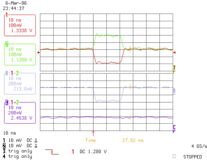
The top two traces are the output LVDS levels, the third trace is the difference of the two, and the bottom trace is the sum, or 2x the common mode level. A proper LVDS signal from the ASD should have a differential swing of 400mv and a common mode swing of zero. Note that the pulse width is ~20ns and is controlled by the setting of the Wilkinson gate width. With zero hysteresis setting, about 85% of the noise pulses look like the traces above.
