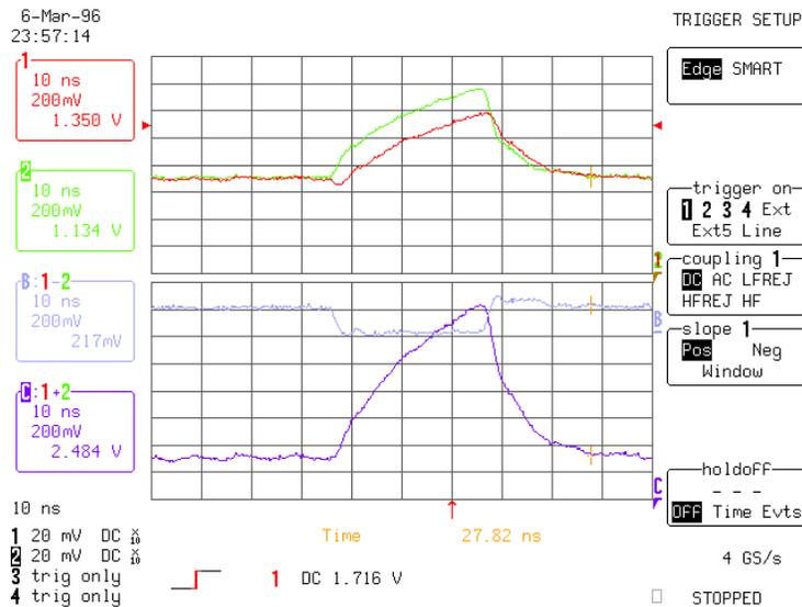
Note that in the above case, the differential signal is only half its expected size and there is a common mode swing of about 0.5 volts. The root of this phenomenon certainly
