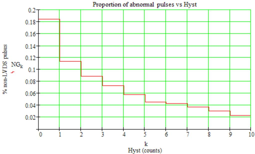
As shown in the above plot, adding hysteresis does not eliminate the abnormal pulses, but it does reduce their frequency from 18% with no hysteresis down to about 2% with 10 counts or 15mv. Note that hysteresis produces symmetrical threshold shifts which must be subtracted from the threshold setting. So, for example, if we wish to use five counts of hysteresis, the threshold must be reduced by  $5 \times 1.5\text{mv} = \sim 8\text{mv}$ .
