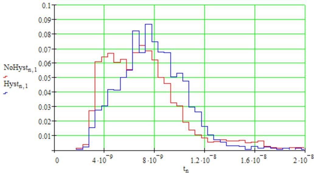
This distribution is about as expected. Adding a few counts of hysteresis has the effect of increasing the peak of the distribution and reducing the number of very narrow pulses. The actual pulse shape of the LVDS signal is also as expected.
