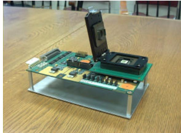
Each ASD chip is serialized before testing with a 2D barcode sticker before loading in the tester. No chip loader robot is used; the test socket is loaded and unloaded manually by technicians. The overall average test rate was 2.5 devices/minute. A total of 72,000 devices were tested in 3 months on one test station.
