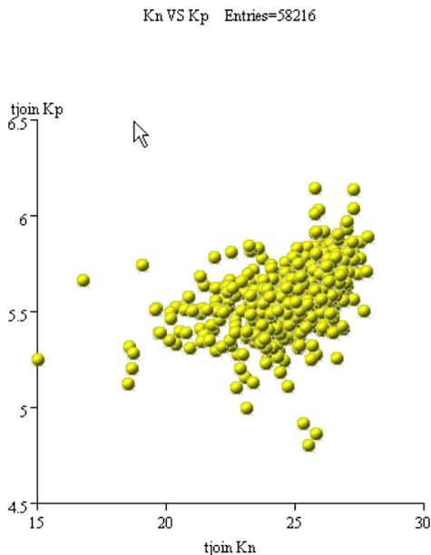
An interesting bonus is the ability to identify mezzanine boards and (to a certain extent) ASD chips by their “signature” of threshold offsets as stored in the database. By performing a *Monte Carlo* analysis based on stored offset data, it can be shown that any individual mezzanine board can be identified with 99.999% accuracy by an *in situ* threshold sweep measurement after installation.
