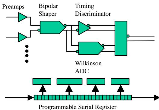
Each ASD channel begins with two identical transimpedance preamplifiers with a gain of about 1mV/fC.
