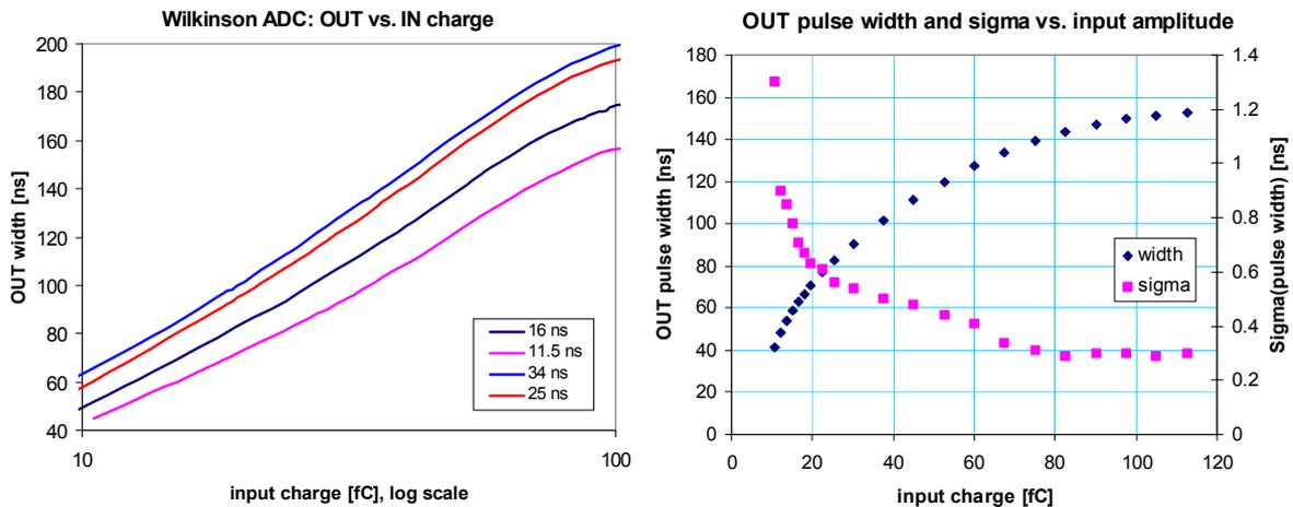
**Figure 40.** Width of the Wilkinson ADC output pulse as a function of input charge for 4 different integration gate widths (left) on a logarithmic scale. The right plot shows the output pulse width (on a linear scale) and the sigma of the width also as a function of the input signal.
