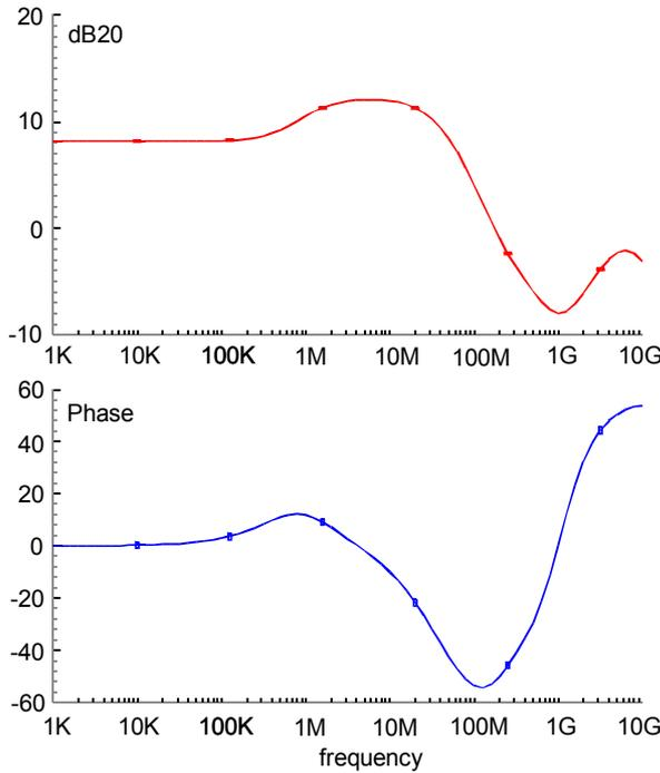
**Figure 16.** DA2 AC characteristics. The voltage gain peaks at ~ 11dB @ 5 – 10 MHz, the roll-off slope is -18dB/octave.
