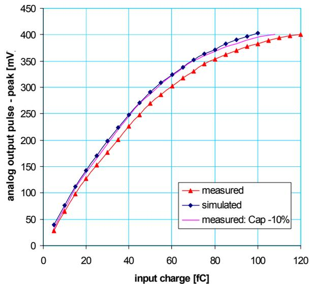
**Figure 27.** Simulated and measured analog output pulse peak versus input charge using the calibration injection system. The blue solid line represents measurement results assuming the on-chip calibration capacitors being 10% lower than their designed value.
