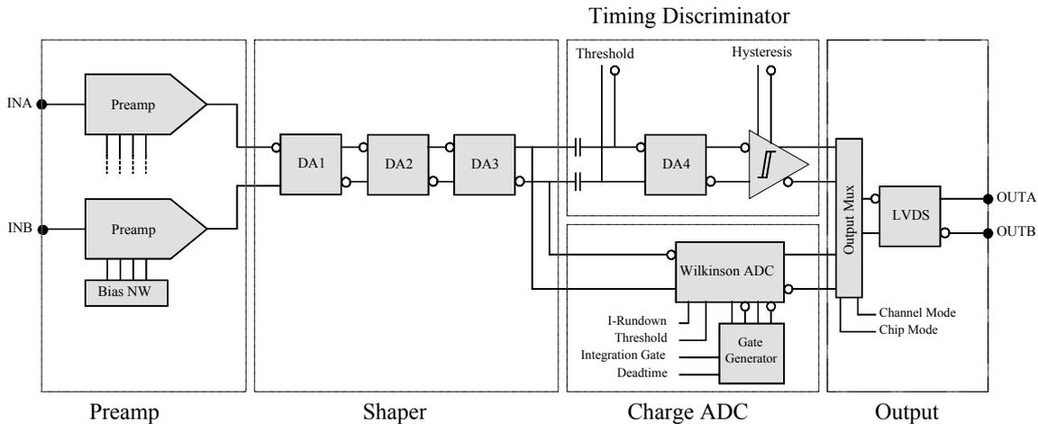
Figure 1. MDT-ASD channel block diagram
