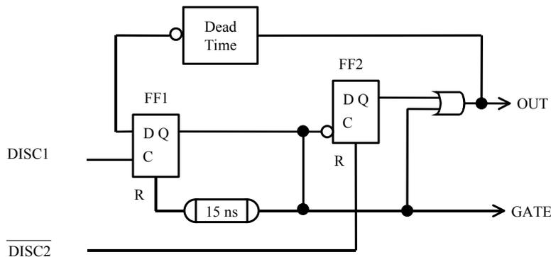
**Figure 9.** Gate generator block diagram
