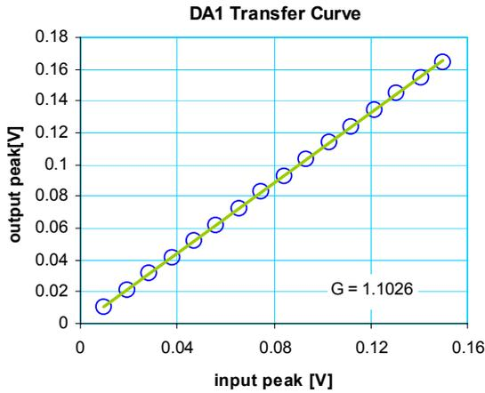
**Figure 12.** Differential amplifier DA1: Output versus input pulse peak voltage. The linear region extends the working signal range by at least a factor of two.
