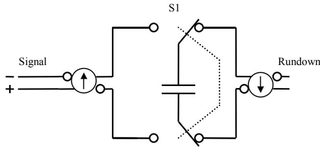
**Figure 8.** Wilkinson charge-to-time converter principle
