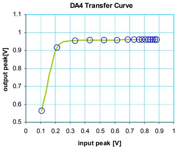
**Figure 18.** Differential amplifier DA4: Output versus input pulse peak voltage (double dynamic range).
