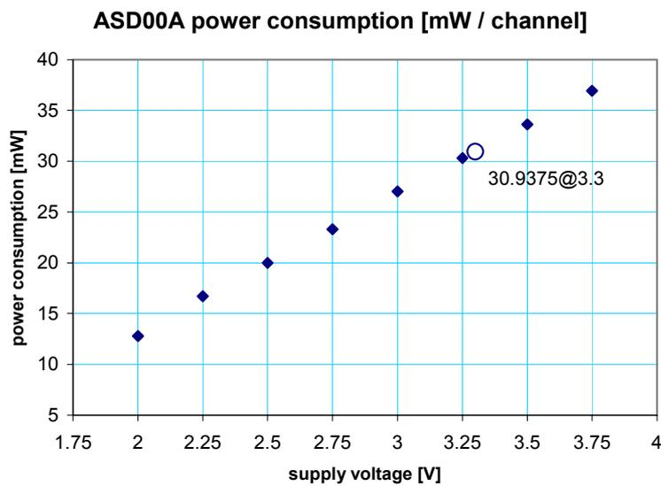
Figure 45. Power consumption versus supply voltage for one channel of the octal ASD00A prototype. The consumption is  $\sim 31 \text{ mW / channel}$  which is in good accordance with the simulated value and slightly below specification (33 mW).
