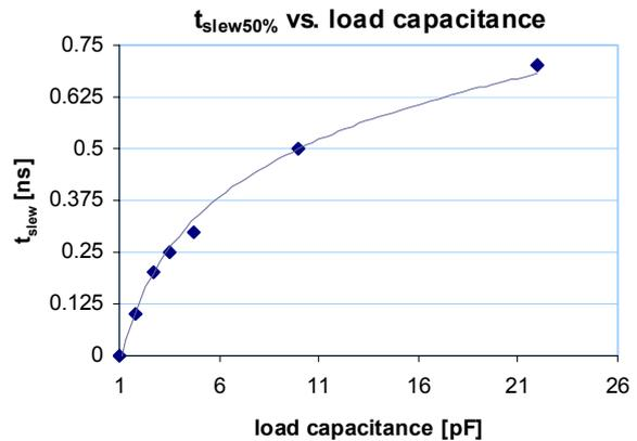
Figure 57.  $t_{slew50\%}$  vs. load capacitance
