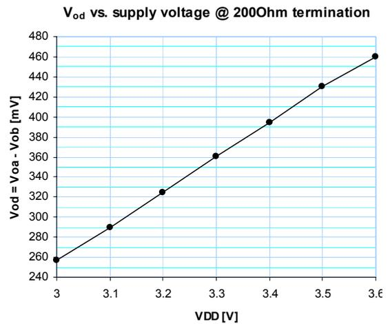
Figure 49. Driver differential voltage vs. supply voltage at 200  $\Omega$  load
