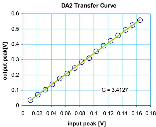
**Figure 14.** DA2 output peak voltage vs. input peak voltage. The voltage gain of 3.4 (10.6dB, compare Figure 16) is linear over the extended dynamic range.
