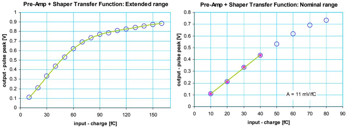
**Figure 20.** Analog signal chain transfer characteristics: Extended (left) and nominal range (right). The linearity within the nominal range is adequate. The sensitivity of the pre-amp – shaper combination is 11 mV/fC.
