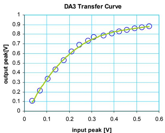
**Figure 15.** DA3 output peak voltage vs. input peak voltage. The small signal voltage gain is ~ 3.2 (~ 10dB, compare Figure 17). The transfer curve shows a compressive characteristic.
