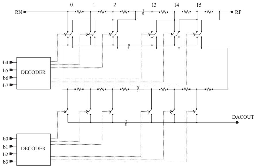
Figure 28. Block schematic of the 8-bit main discriminator threshold voltage DAC
