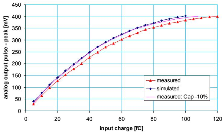
**Figure 35.** Simulated and measured analog output pulse peak versus input charge using the calibration injection system. The blue solid line represents measurement results assuming the on-chip calibration capacitors being 10% lower than their designed value.
