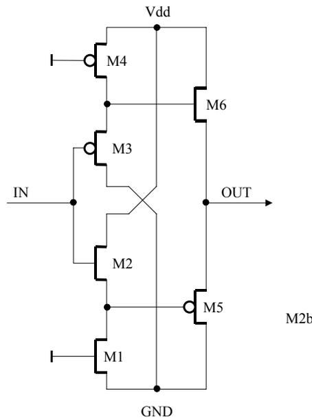
Figure 7. Analog pad driver simplified schematic
