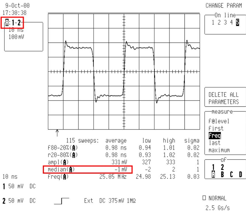
Figure 54.  $|\Delta V_{od}| = 2 |\text{median}(A)| = 2 \text{ mV}$
