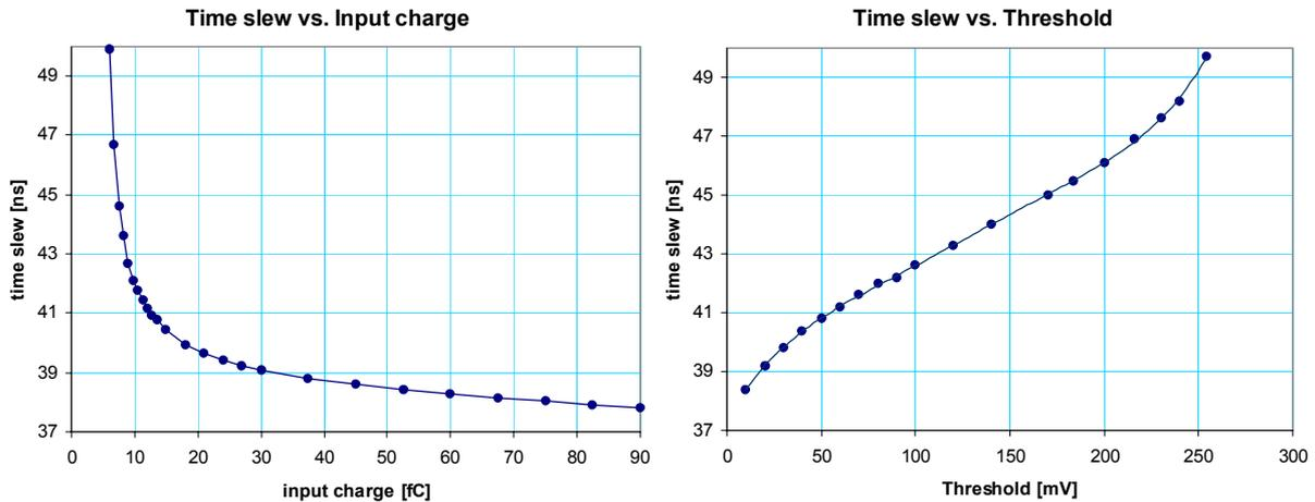
**Figure 39.** Time slew of the MDT-ASD signal chain. The slew is the timing of the discriminator 50% point of transition as a function of input signal amplitude (left) for a 20 mV threshold and as a function of the threshold (right) for a 27 fC input signal.
