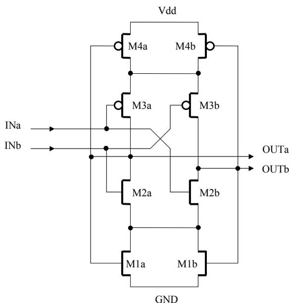
Figure 6. LVDS driver simplified schematic
