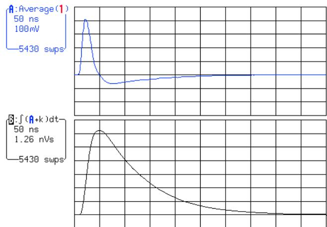
**Figure 36.** Shaper signal and integral
