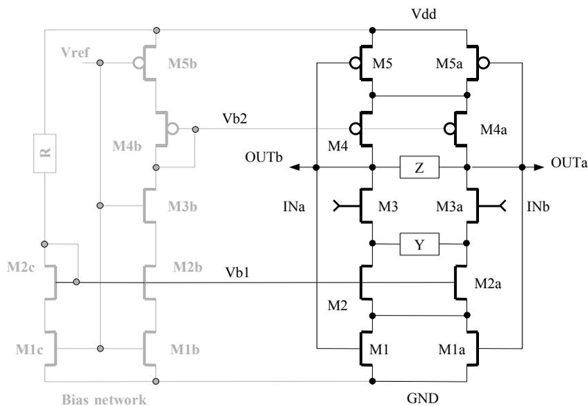
**Figure 3.** Differential amplifier schematic
