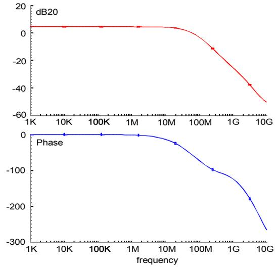
**Figure 13.** Differential amplifier DA1 frequency response – gain and phase Bode plots: The amplifier shows a small signal gain of 4.5dB with the -3dB point at 45 MHz. The rolloff slope is -6dB/octave. The phase plot shows an initial phase shift of 0°, decreasing to -180° at ~ 3 GHz.
