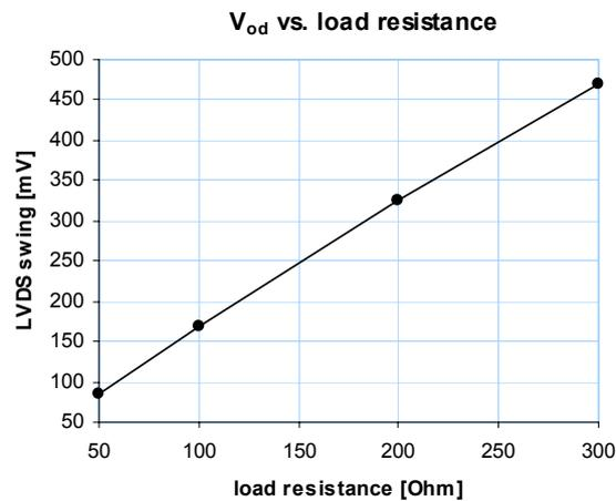
Figure 50. Driver differential voltage vs. load resistance
