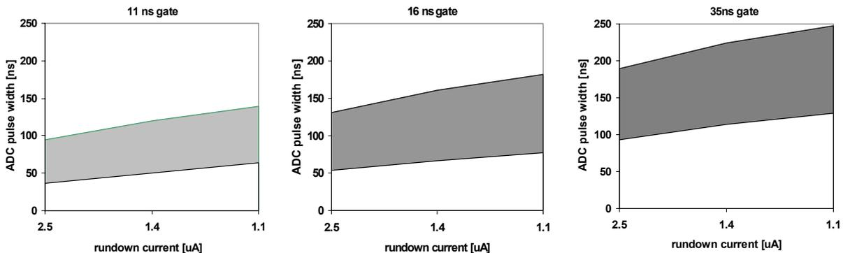
Figure 30. Influence of integration gate and rundown current settings on the ADC output pulse width.
