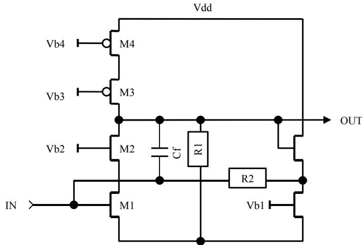
**Figure 2.** Pre-amp simplified schematic
