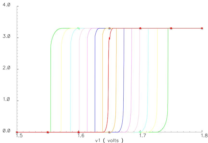
Figure 29. Simulation of the timing discriminator output vs. input voltage DC sweep for the eight different Hysteresis-DAC settings
