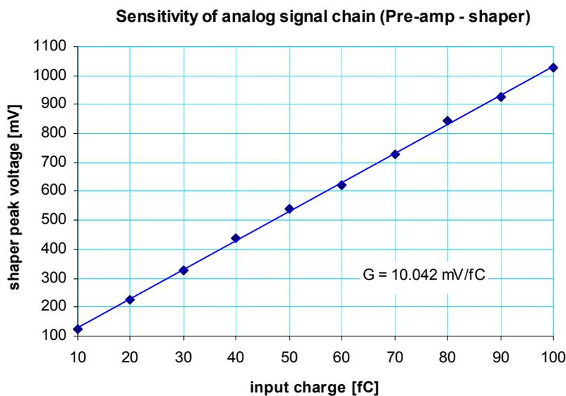
**Figure 38.** Sensitivity of the analog signal chain (Pre-amp to shaper) for the expected input signal range. The gain amounts to ~ 10 mV/fC, exhibiting very good linearity.
