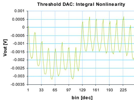
**Figure 43.** VDAC integral non-linearity
