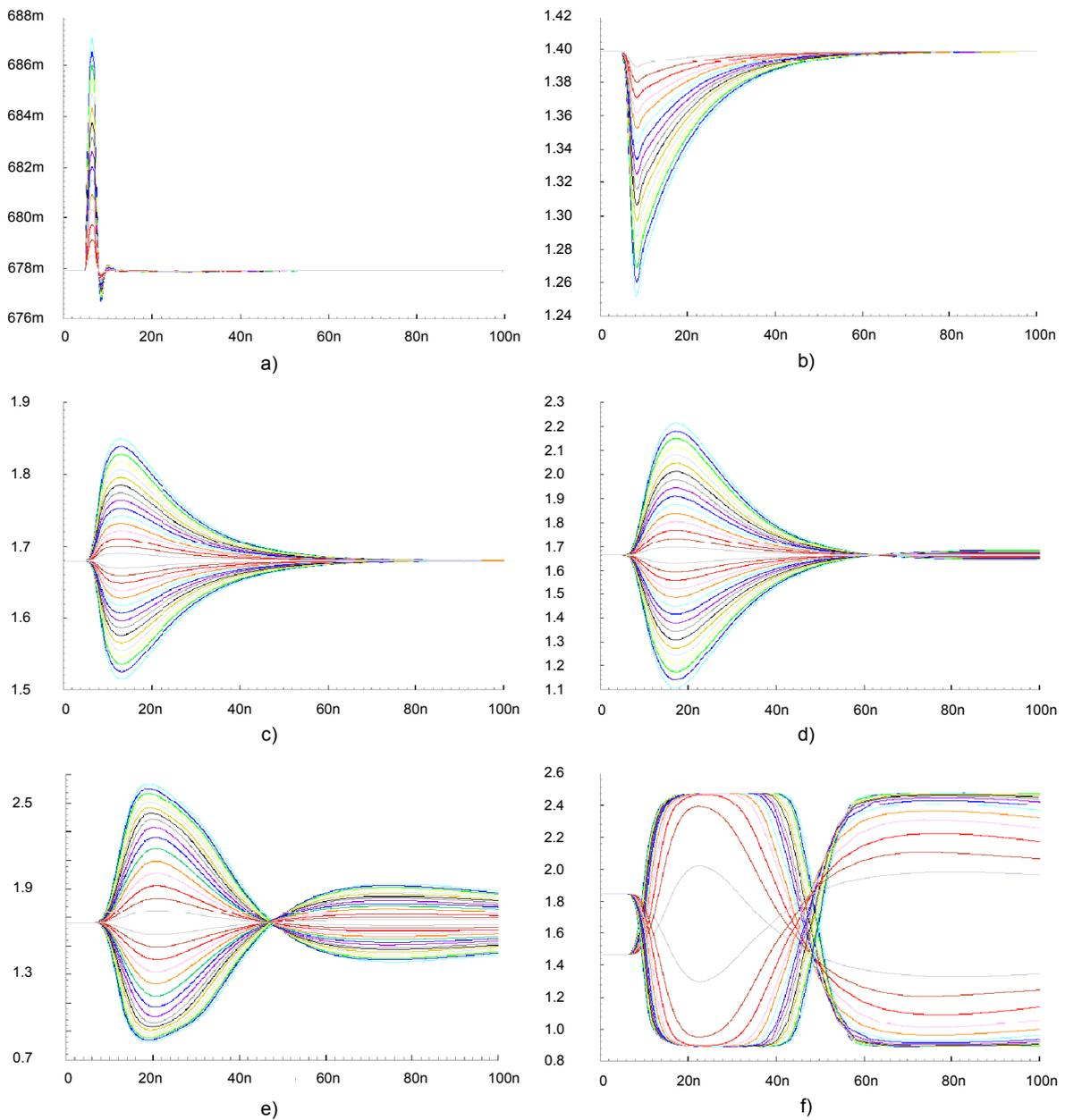
**Figure 22.** Spice simulation of the Delta pulse (a) response of the analog signal chain after the pre-amp (b), DA1 (c), DA2 (d), DA3 (threshold coupling point) (e) and DA4 (pre-discriminator gain stage) (f).
