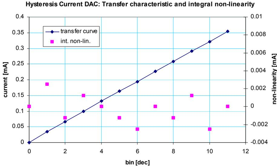
Figure 44. Hysteresis DAC transfer curve and integral non-linearity.
