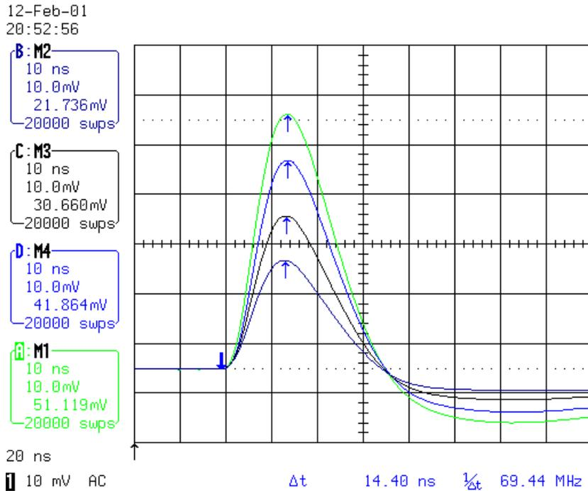
**Figure 37.** Shaper output for 40, 60, 80 and 100 fC input charge. The peak voltages translate into the sensitivity curve below (Figure 37) by multiplying with a factor of two (single-ended to differential) and including a probe attenuation of 10:1.
