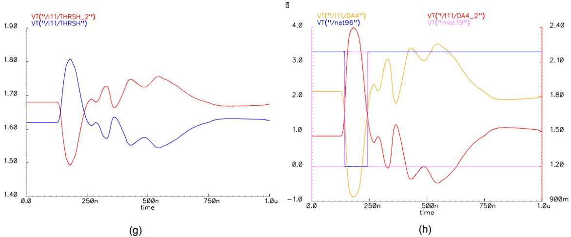
Figure 23. Response of one ASD channel to a MDT current signal created by GARFIELD [10].
