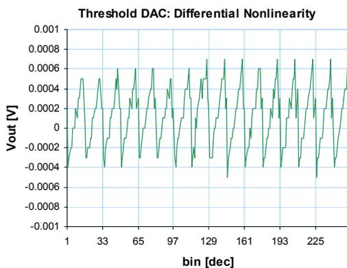
**Figure 42.** VDAC differential non-linearity
