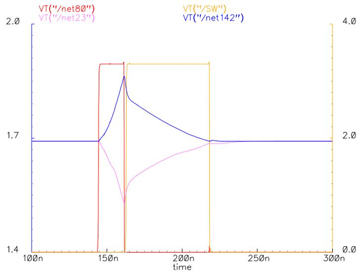
**Figure 25.** Wilkinson ADC: Internal ramp signals and gate signals (integration gate and rundown gate). The ADC output pulse is constituted by the OR disjunction of the two gate signals.
