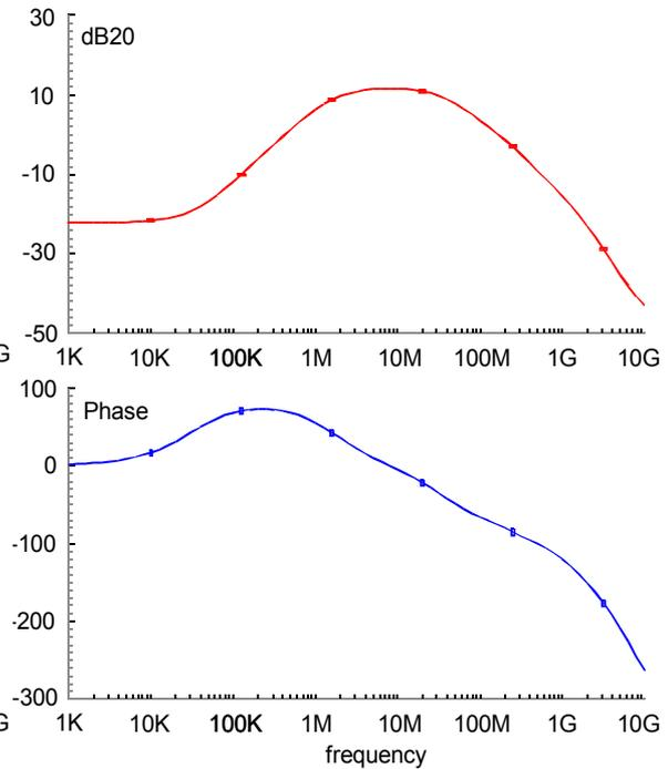
**Figure 17.** DA3 AC characteristics. The voltage gain peaks at ~ 10dB @ 5 – 10 MHz, the roll-off slope is -12dB/octave.
