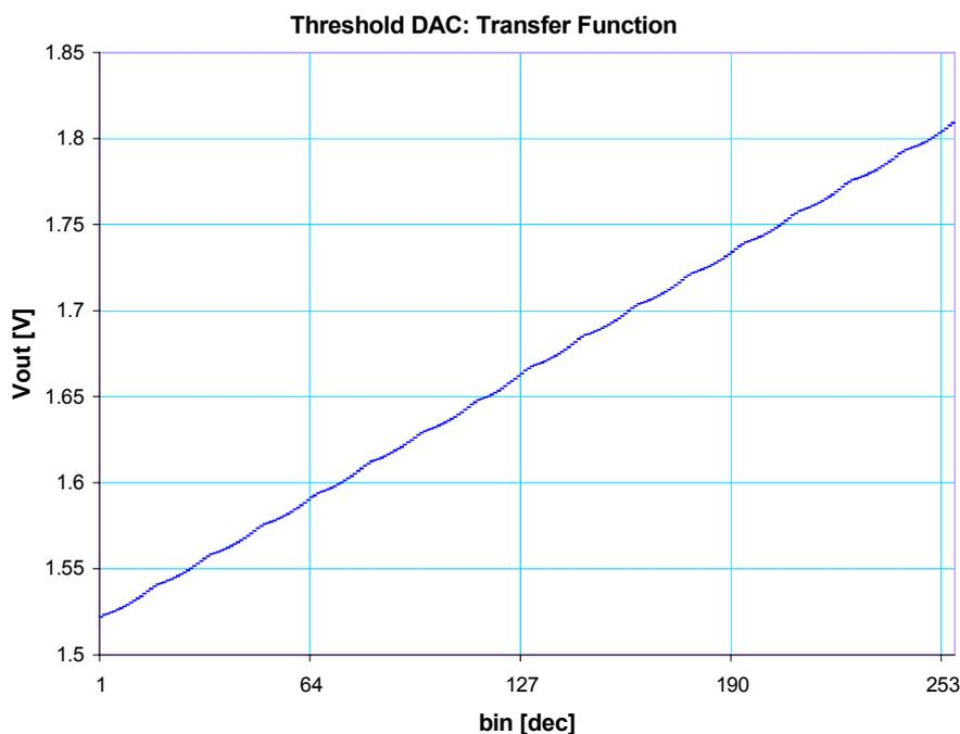
**Figure 41.** VDAC transfer function
