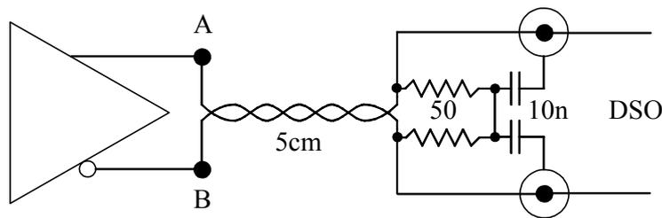
Figure 52. Connection setup: 5cm twisted pair terminated with  $50 \Omega$  resistors, 10nF caps to scope ground.
