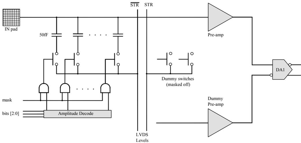
Figure 31. Calibration/test pulse injection – block diagram
