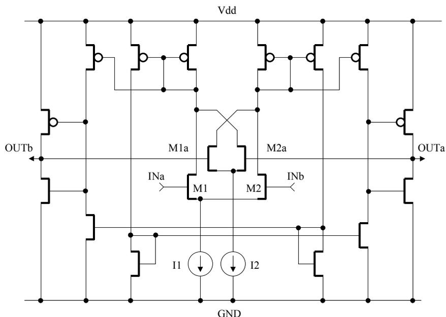
Figure 5. Discriminator simplified schematic
