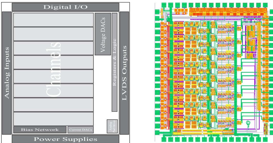
Figure 34. Octal MDT-ASD: Floor plan and chip layout for the HP  $0.5\ \mu\text{m}$  CMOS process
