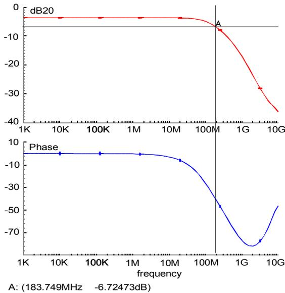
**Figure 26.** Analog pad driver frequency response – gain and phase Bode plots: The amplifier shows a small signal gain of  $-3.7\text{dB}$  with the  $-3\text{dB}$  point at  $184\text{ MHz}$ . The rolloff slope is  $-6\text{dB/octave}$ .
