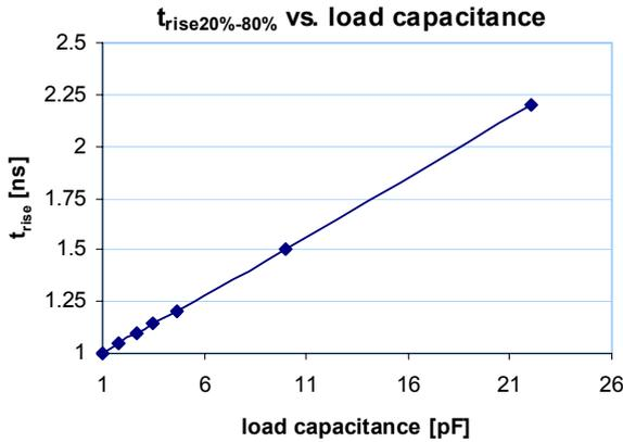
Figure 56.  $t_{rise}$  vs. load capacitance
