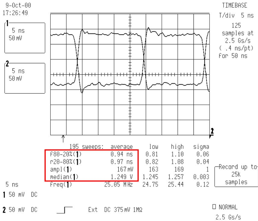
Figure 53.  $t_{rise}$  and  $t_{fall}$ ,  $V_{od} = \text{ampl}(1)$ ,  $V_{os} = \text{median}(1)$
